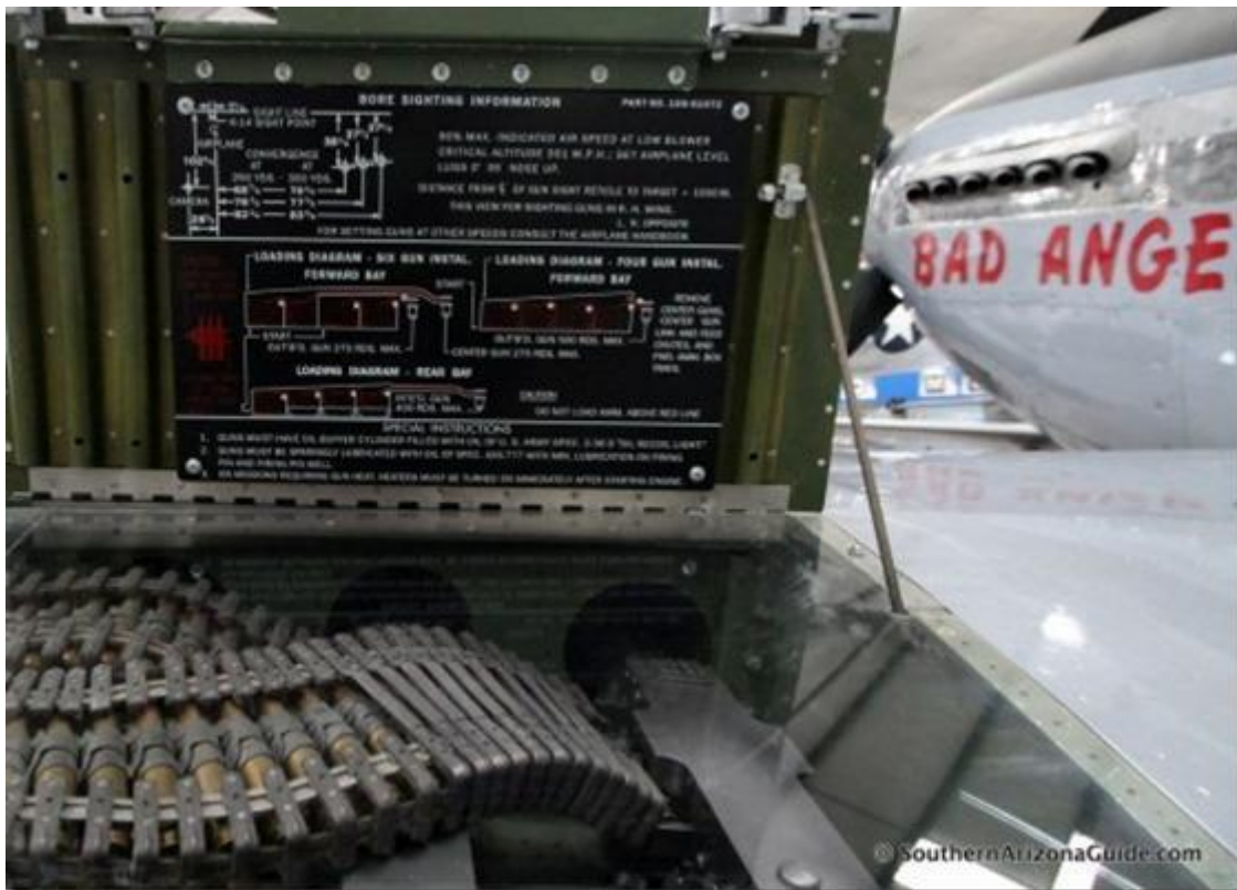
One of "Bad Angel's" .50 caliber machine guns built into it wings.
